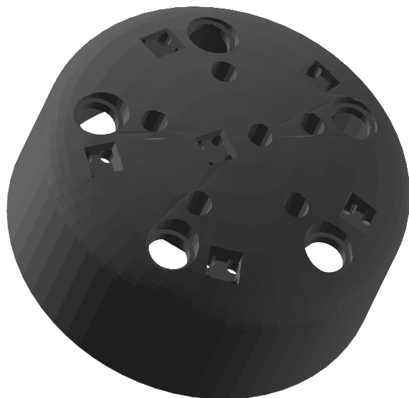
Figure 3: The final design of the casing for each node, rendered with SolveSpace [75].
